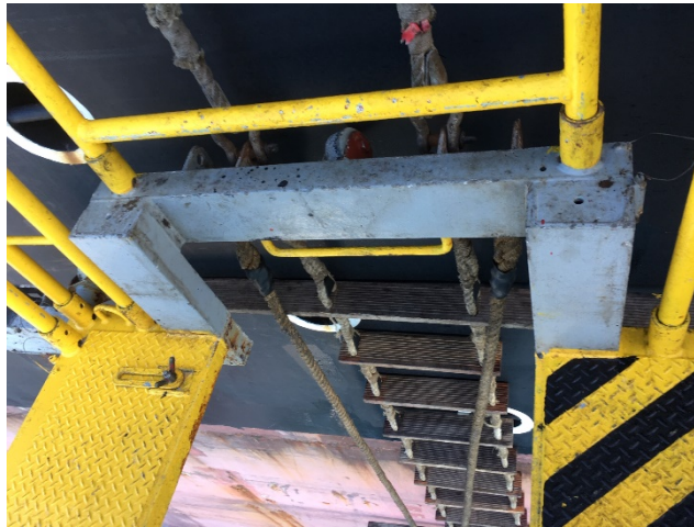
Figure 9 – Pilot has to lean back to gain access to trapdoor
