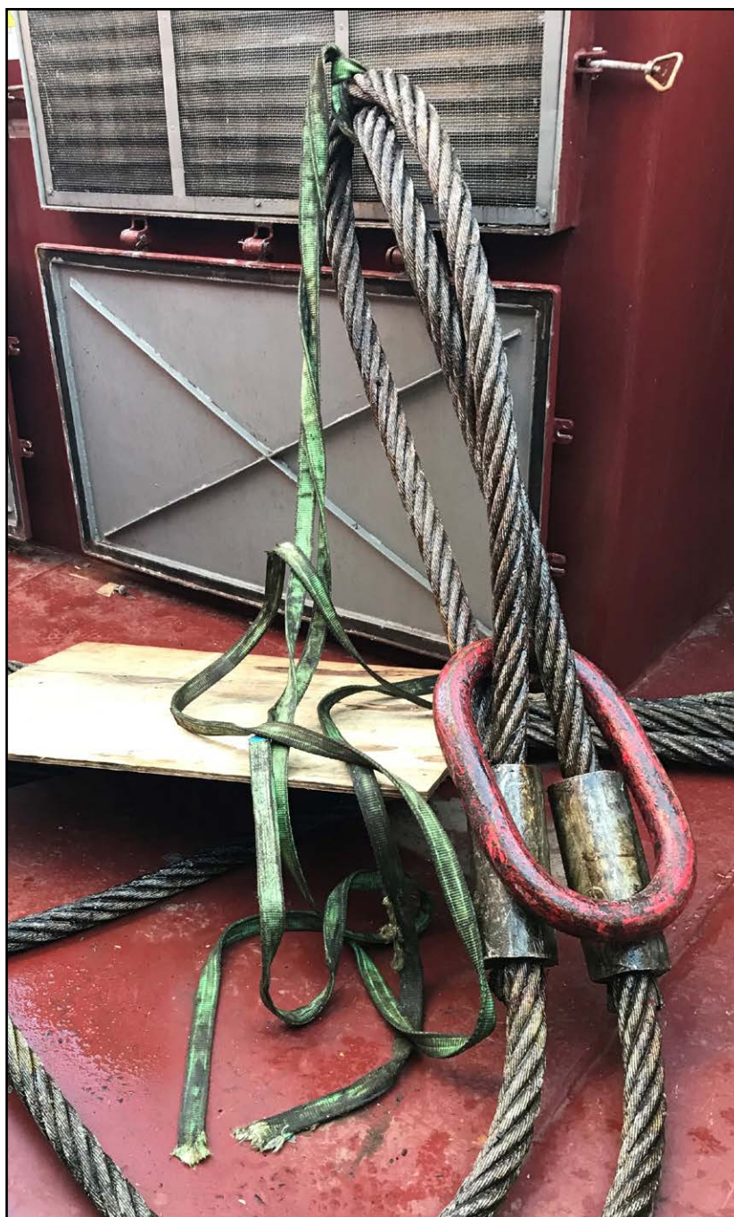
Figure 4: Broken fibre sling (after the accident)
