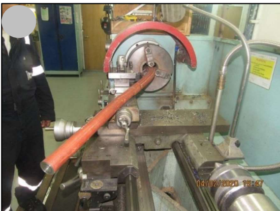
Figure 3: Condition of rod after accident
