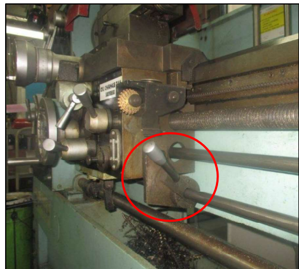
Figure 5: Spindle control lever in lifted position
