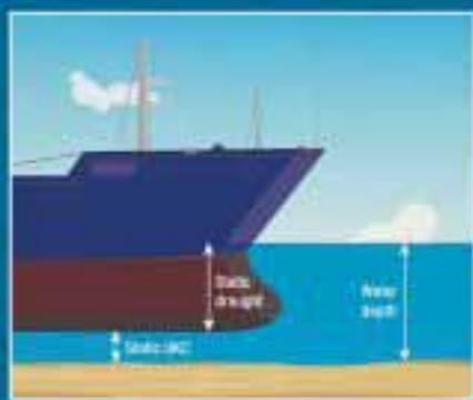
◀ Figure 1 – Static UKC: static draught is taken to be the maximum of fore and aft draughts
