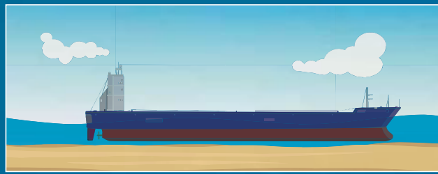
▶ Figure 4 – Panamax bulk carrier in head seas. Wave period is 12 seconds and wave height is 4m. Draught is 12.2m, water depth is 14m and bow is close to grounding
