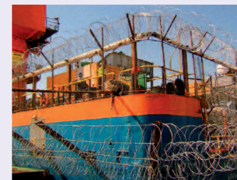
Vessel security hardening at Jebel Ali
